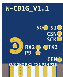
Figure 4. W-CB1G 测试点定义
